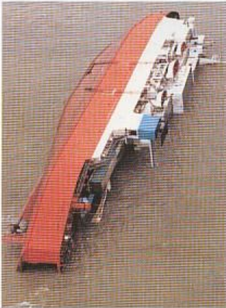
A Ro-Ro ship which has capsized due to the free surface effect
