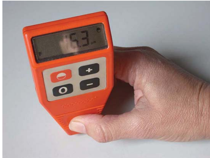
Photograph 8-9. Dry Film Thickness Gauge.
