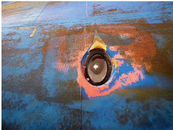
Photograph 6-7. An example of an ICCP anode on a ship.
