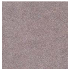
C HB 2.5 Rust Grade C Hydroblasted to an Sa 2.5 equivalent
