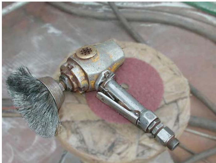
Photograph 4-7. Rotary wire brush.
