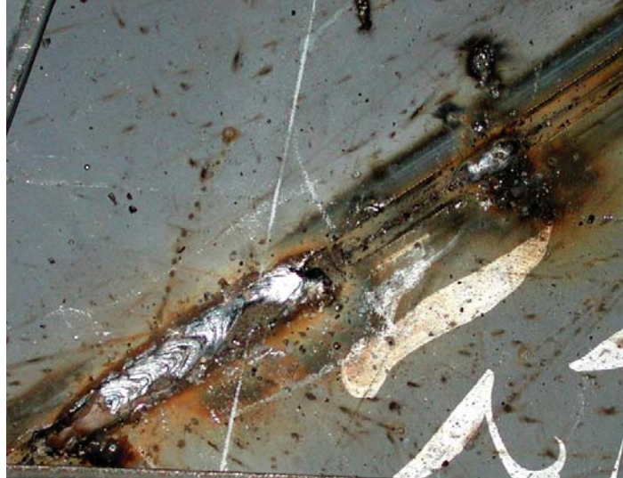
Photograph 4-9. Weld fume (brown stains) & spatter.
