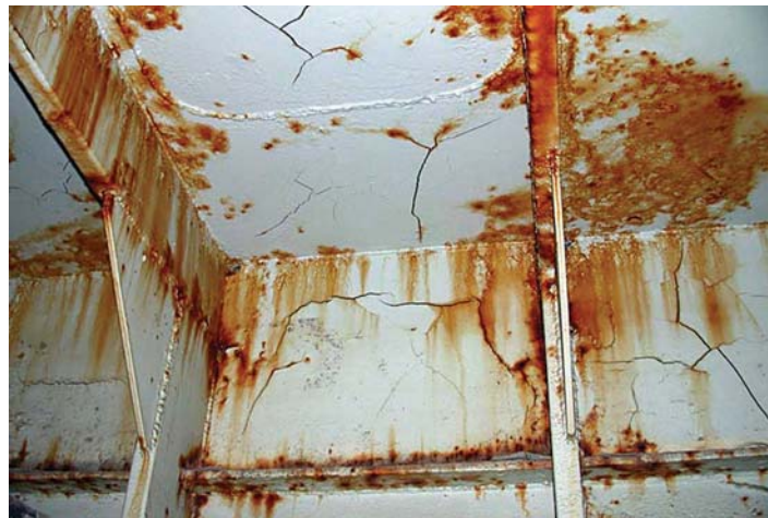
Photograph 12-24. Mud cracking of a very thick coating.
