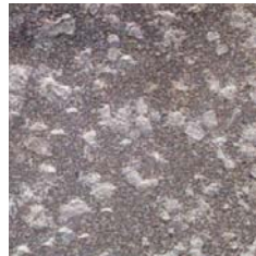
D HB 2.5 Rust Grade D Hydroblasted to an Sa 2.5 equivalent
