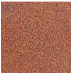
Rust Grade C
