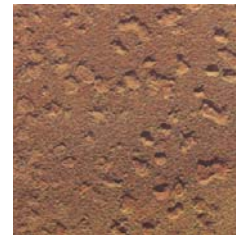
D HB 2.5 H Heavy Flash Rusting
