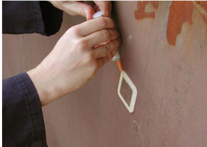
Photograph 8-7. Bresle patch test for soluble salts.
