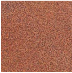
Rust Grade C
