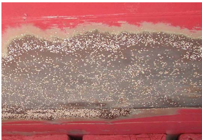
Photograph 7-2. Early stages of barnacle fouling on an area where the anti-fouling paint has been damaged.
