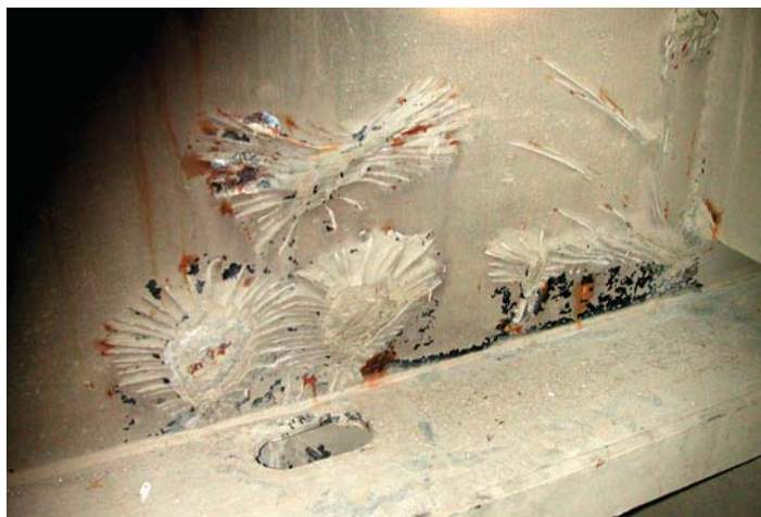
Photograph 12-21. Reverse impact from grab causing brittle coating to shatter.
