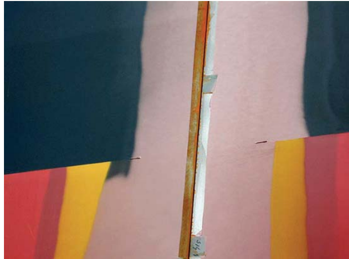
Photograph 8-5. Feathered paint layers on an outer hull.
