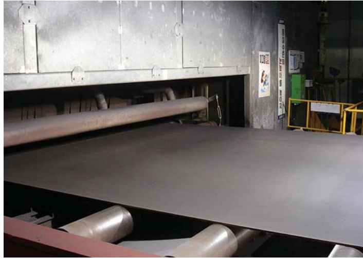
Photograph 8-1. Steel plate after blasting on the shop primer line.
