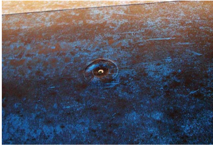
Photograph 6-6. An example of a zinc reference electrode on a ship.
