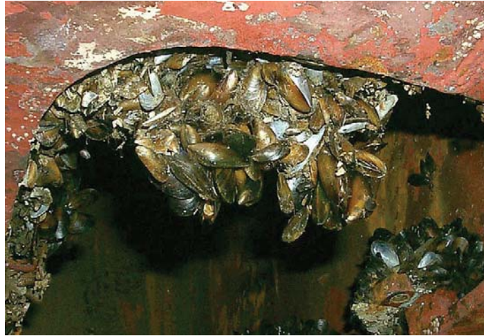
Photograph 7-3. Mussel fouling in a sea chest.
