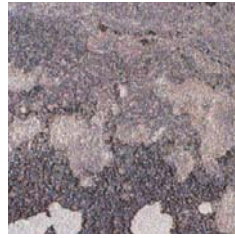
D HB 2 Rust Grade D Hydroblasted to an Sa 2 equivalent
