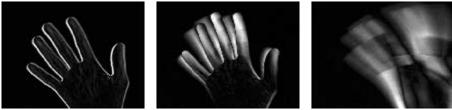
Example 1. Detects motion by comparing each video frame to the previous frame. The change is visualized and is calculated as a number.
